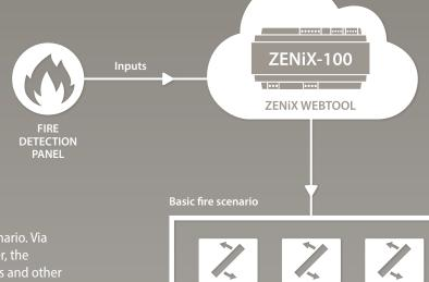
The ZENiX-100 controller is supplied with an onboard pre-programmed fire scenario. Via one or two physical inputs on the controller, the scenario can be triggered, and the dampers and other components can be brought to their safety position. No programming is required, only cabling and connection to the output (alarm) of the fire alarm system.
