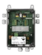
The ZENiX 2MFD field device is used to monitor up to 2 mechanical (fusible link) dampers. No configuration is required as it has a predefined device address.
