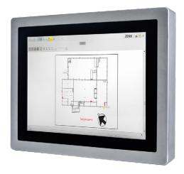
easy to navigate virtually through the building. The panel PC has a full IP65 casing and can easily be placed on a wall, for example, in a technical room.
