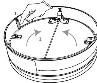
2. Press the two blocking hooks carefully to unlock the blades.
