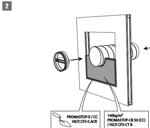
2. The opening in the wall around the duct in which the fire damper cartridge is mounted, is sealed with 2 layers of 50 mm-thick stone wool panels with fire resistant coating on one side (type PROMASTOP-CB 50 / PROMASTOP-CB/CC 50 / HILTI CFS-CT B).
