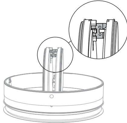
2. Unlock (close) the damper blades by pushing them towards each other. Carefully unlock the fusible link by pushing it sideways.
