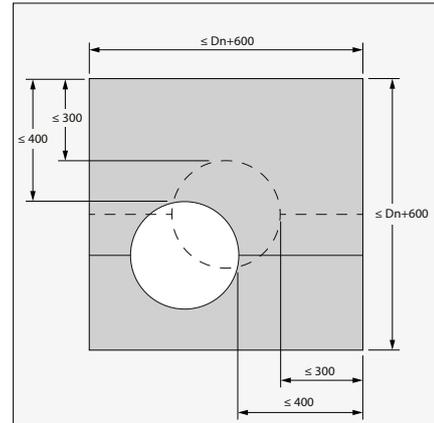
8. The duct in which the damper is inserted doesn't need to be centered in the opening (with max dimensions duct + 600 mm). The maximal distance between the damper and the edge of the opening is 425 mm.
