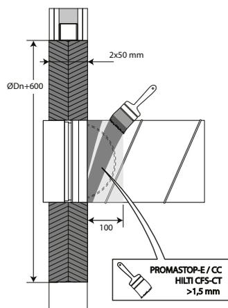
5. The duct is coated with a layer (>1,5 mm) of endothermic coating (type PROMASTOP-E / PROMASTOP-CC / HILTI CFS-CT) on a width of 100 mm at the side the open damper blade exceeds.
