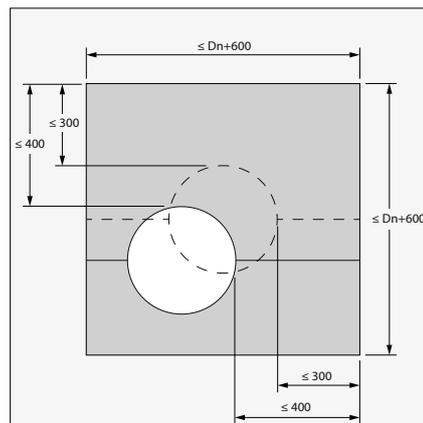
6. The duct in which the damper is inserted doesn't need be centered in the opening (with max dimensions duct + 600 mm). The maximal distance between the damper and the edge of the opening is 400 mm.
