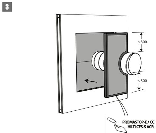
3. The joints on these 2 layers must be installed staggered and covered all around the edge with coating (type PROMASTOP-E / PROMASTOP-CC / HILTI CFS-S-ACR).
