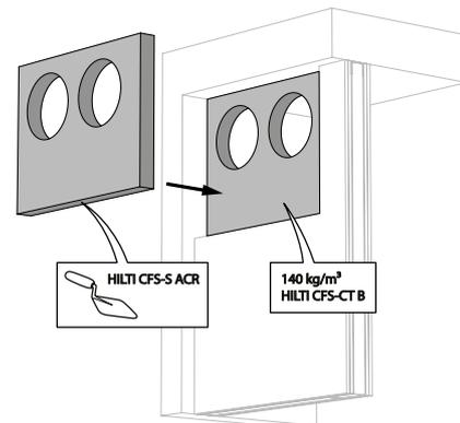
3. The opening in the wall around the duct in which the fire damper cartridge is mounted, is sealed with 2 layers of 50 mm-thick stone wool panels with fire resistant coating on one side (type HILTI CFS-CT B).
