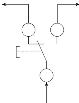
1. An end of range switch (FCU) can be mounted on the metal body. The purpose is to determine the position of the circular fire damper cartridge from a distance. 1mA...6A DC 5V... AC250V.
