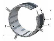
The fire resistant collar MG-U is suitable for installation around ventilated and non-ventilated plastic pipes (PVC, HDPE, PP, ABS, SAN+PVC). The MG-U is cast in the wall or floor in order to prevent propagation of fire for up to 120 minutes.
