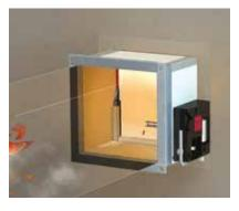
A fire breaks out and the temperature reaches 72°C: the fusible link melts and the damper blade closes.
