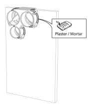
6. Seal the rest of the opening with standard mortar or gypsum (only for vertical walls).
