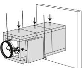
5. The opening around the duct is sealed with standard mortar.
