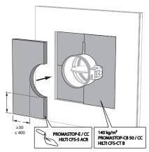
2. The opening around the damper is sealed with 2 hard rock wool slabs of 50 mm. These boards should be placed in a slanted position and the joints should be covered all around with filling paste.
