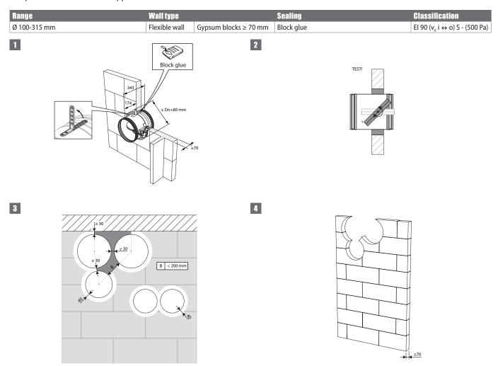
3. The dampers can be installed at a minimum distance from an distance from an 4. Make the necessary openings ( $\leq$  Dn + 80 mm) in the wall. adjacent wall or from another damper.
