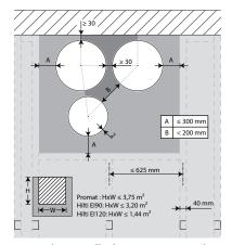
7. The dampers can be installed at a minimum distance ( $\geq$  30 mm) from an adjacent wall or from another damper.
