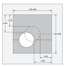
6. The damper does not need to be centered in the opening (with max dimensions fire damper + 600 mm). The maximal distance between the damper and the edge of the opening is 400 mm.
