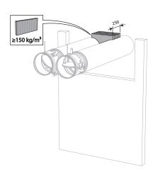
10. Apply rigid stone wool panels (150 kg/m³) to a depth of 250 mm (wall thickness + additional at the rear side of the wall) to seal the opening at the side with minimal distances. When the distance between the damper and the wall is greater than 75 mm, the sealing of the opening between the damper and the wall is carried out according to the pre-existing classification.
