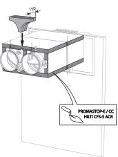
13. Apply rigid stone wool panels (150 kg/m³) to a depth of 150 mm to seal the opening at the side with minimal distances.
