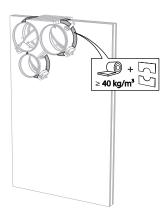
8. Seal the rest of the opening with standard stone wool 40 kg/m<sup>3</sup> across the entire wall thickness.
