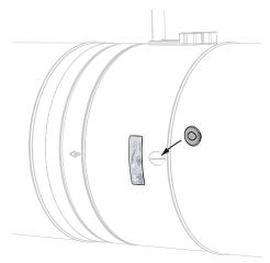
3. After inspection, replace the air-tight plug thoroughly on the damper opening. The position is crucial in order to maintain the air-tightness of the fire damper.
