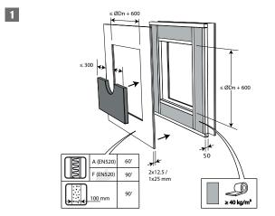
1. The opening around the damper is sealed with 2 layers of 50 mm-thick mineral wool panels with fire resistant coating on one side (type PROMASTOP-CB 50 / PROMASTOP-CB/CC 50 / HILTI CFS-CT B / Mulcol Multimastic FB1 / PYRO-SAFE® MFP).
