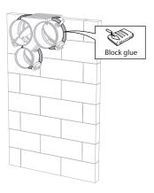
6. Seal the rest of the opening with block glue across the entire wall thickness.
