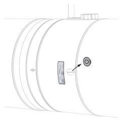
1. Remove the air-tight plug from the damper.
