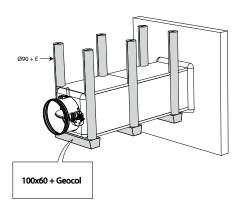
7. The threaded rods are covered with U-shaped plates of GEOFLAM (Ø 90 mm) and affixed with glue and fibrous plaster. The profiles are covered with U-shaped shells GEOFLAM 100 x 60 mm, which are affixed to the underside of the shaft with GEOCOL (GEOSTAFF) cement plaster.
