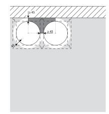
8. The dampers can be installed at a minimum distance from an adjacent wall or from another damper.
