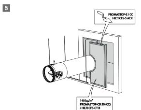
5. The opening around the duct is sealed with stone wool plates type Promastop CB(/CC) / Hilti CFS-CT B ("G"). The edges are sealed and maintained in place with PROMASTOP E / PROMASTOP CC / HILTI CFS-S ACR coating.
