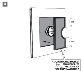
3. The joints on these 2 layers must be installed staggered and covered all around the edge with coating (type PROMASTOP-E / PROMASTOP-CC / HILTI CFS-S-ACR / Mulcol Multimastic SP / PYRO-SAFE® FLAMMOTECT-A).
