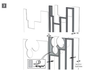
7. Build the drywall and foresee horizontal and vertical studs around the opening.
