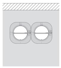
6. The dampers can be installed at a minimum distance from an adjacent wall or from another damper.
