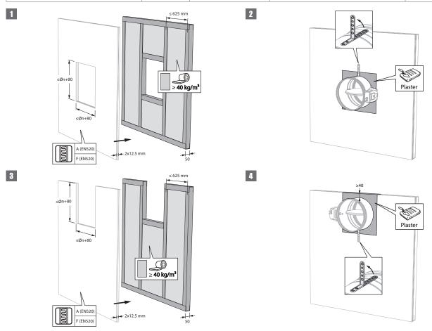
3. The dampers can be installed at a minimum distance (  $\geq$  40 mm) from a ceiling or floor slab.
