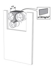
10. Apply rigid stone wool panels ( $\geq$  150 kg/m³) to a depth of 400 mm (150 mm on the mechanism side of the wall) to seal the opening at the side with minimal distances.
