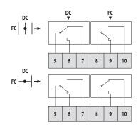
**DC:** Switch open position fire damper **FC:** Switch closed position fire damper
