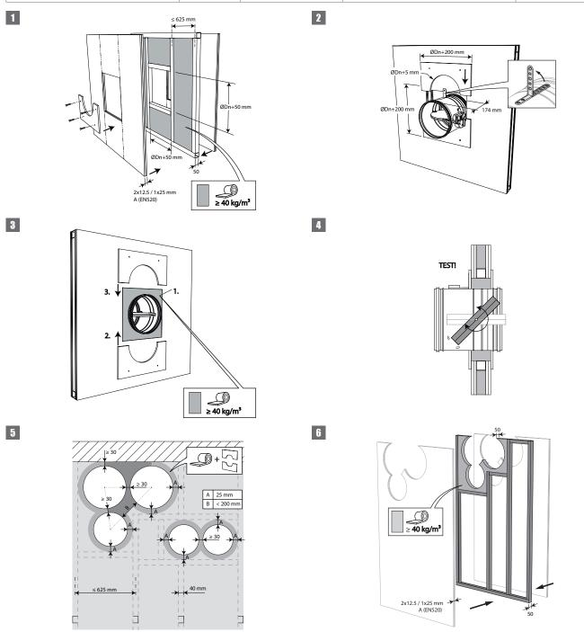
5. The dampers can be installed at a minimum distance (≥ 30 mm) from an adjacent wall or from another damper.
