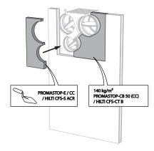
11. Seal the rest of the opening with 2 layers of 50 mm-thick coated rigid mineral wool panels (see above).
