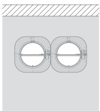
5. The dampers can be installed at a minimum distance from an adjacent wall or from another damper.
