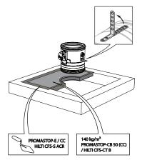
1. The opening around the damper is sealed with 2 layers of 50 mm-thick mineral wool panels with fire resistant coating on one side (type PROMASTOP-CB 50 / PROMASTOP-CB/CC 50 / HILTI CFS-CT B).
