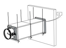
5. The opening around the duct is sealed with standard mortar. The duct is covered with 45 mm thick GEOFLAM F plates or 35 mm thick GEOFLAM Light plates "G".
