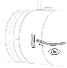
2. Insert the camera of the endoscope (for example Inspecam Rf-t) through the opening and inspect the inside of the damper.
