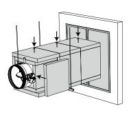
6. The duct is covered over its entire length with stone wool plates "G". To adhere to the duct, the plates are completely coated on one side with fire resitant coating and affixed to the duct with steel screws and washers "E".
