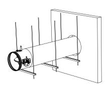
3. An opening with maximal dimensions "A" is made in the wall.
