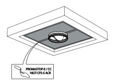
3. The joints on these 2 layers must be installed staggered and covered all around the edge with coating (type PROMASTOP-E / PROMASTOP-CC / HILTI CFS-S-ACR).
