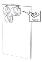
6. Seal the rest of the opening with standard gypsum across the entire wall thickness.
