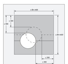
6. The damper does not need to be centered in the opening (with max dimensions fire damper + 600 mm). The maximal distance between the damper and the edge of the opening is 400 mm.
