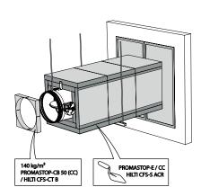
7. An additional stone wool panel type "G", coated with PROMASTOP E / PROMASTOP CC / HILTI CFS-S ACR, is applied in the opening between the damper casing and the stone wool panels.
