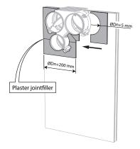
9. Apply cover plates (gypsum plasterboards) to finish the surface at both sides.
