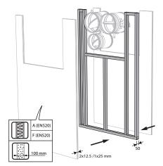
9. Build the drywall and foresee horizontal and vertical studs around the opening.
