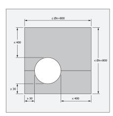
4. The damper does not need to be centered in the opening (with max dimensions  $\emptyset$  fire damper + 800 mm). The maximal distance between the damper and the edge of the opening is 400 mm.
