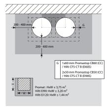
8. The dampers can be installed at a minimum distance from an adjacent wall or from another damper.
